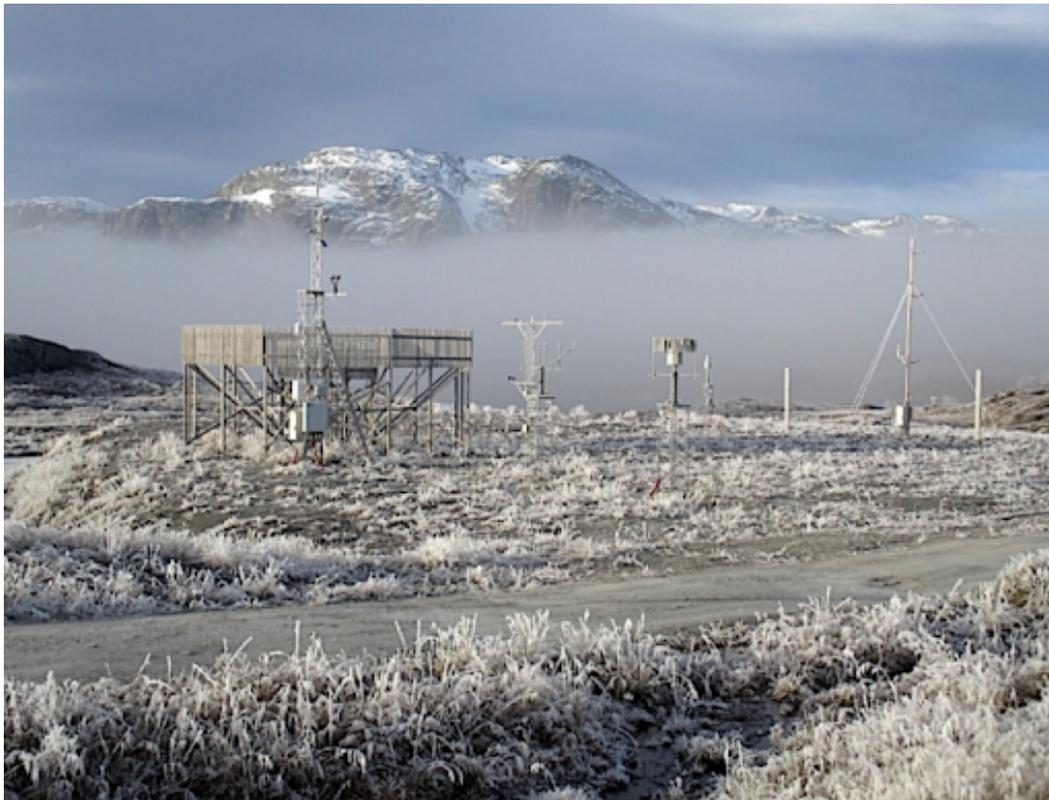
FIGURE 2.5: Photo of the weather instruments at the Haukeliseter site including the Double Fence, one of the single fences, and the tower with the wind and temperature measurements. Courtesy of Claire Pettersen.
